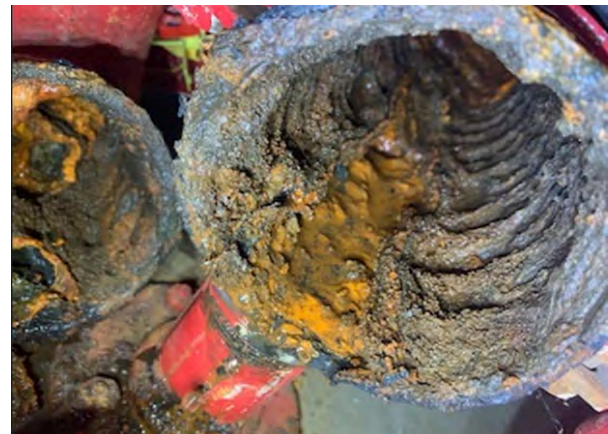
Figure 23. Degraded 222-S Laboratory firewater riser.
