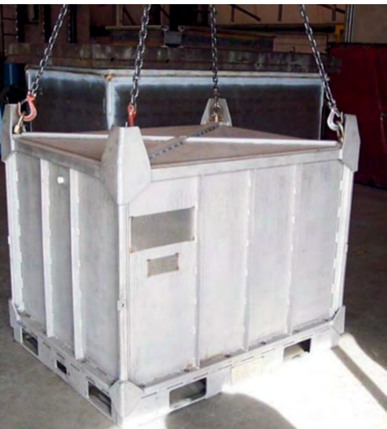
Figure 40. Current shipping container used for subcritical experiments that does not provide protection from fires or electrical insults.
