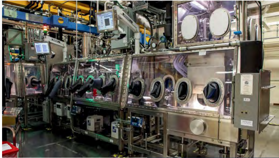
Figure 10. Electrorefining glovebox in the 9215 Complex.
