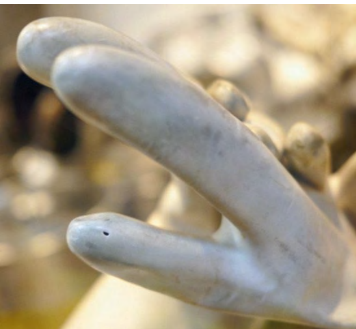
Figure 5. Glovebox glove puncture, risking worker exposure to plutonium.
