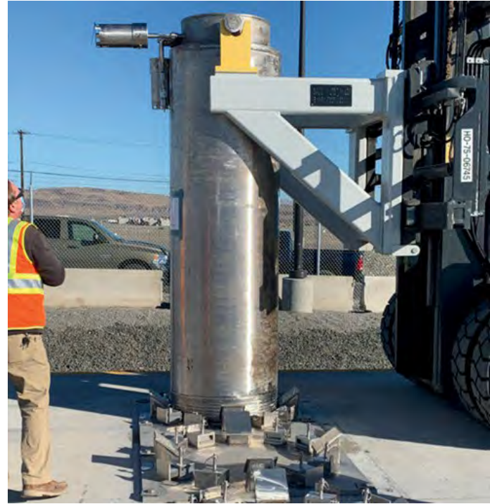
Figure 34. Tank Side Cesium Removal system ion exchange column.
