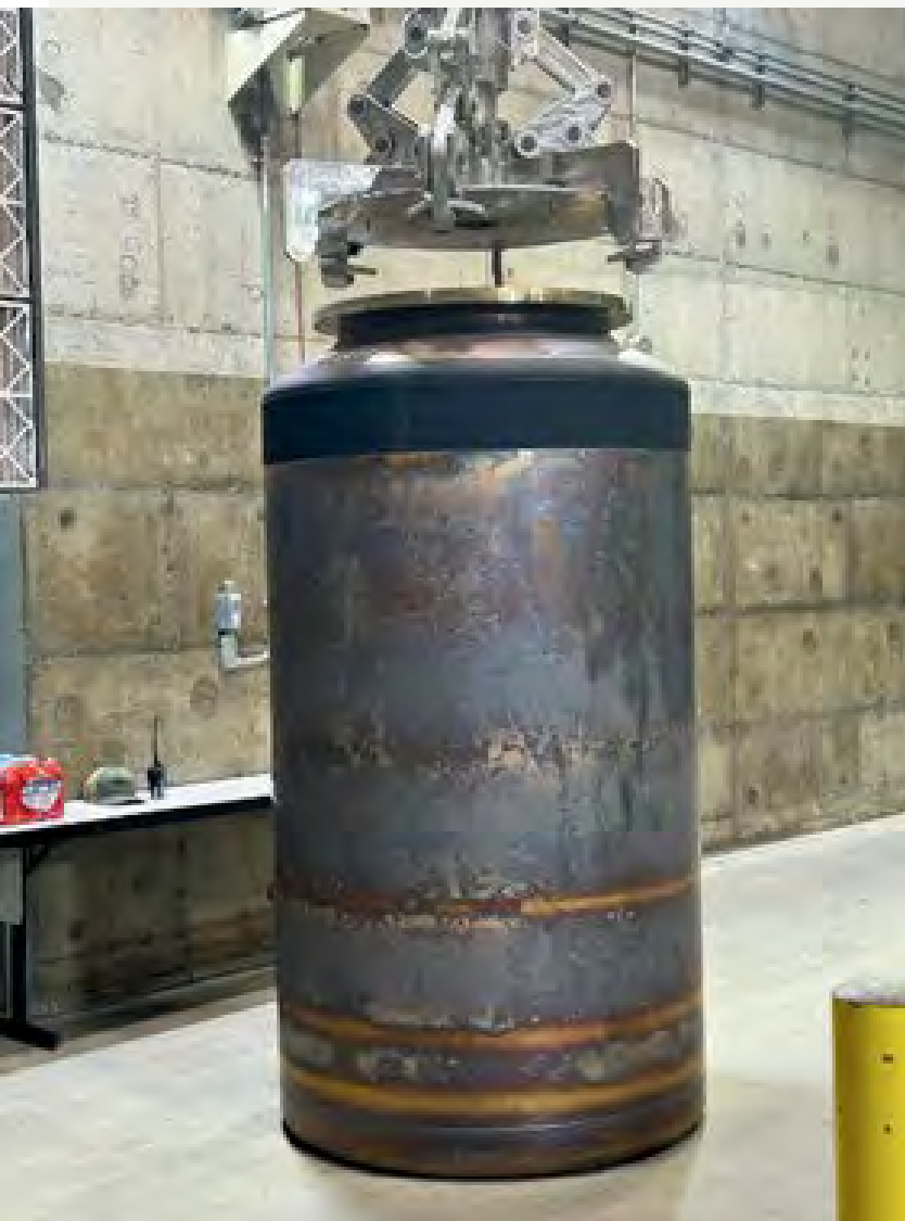
Figure 17. First container of simulated waste produced at the Low-Activity Waste Facility.
