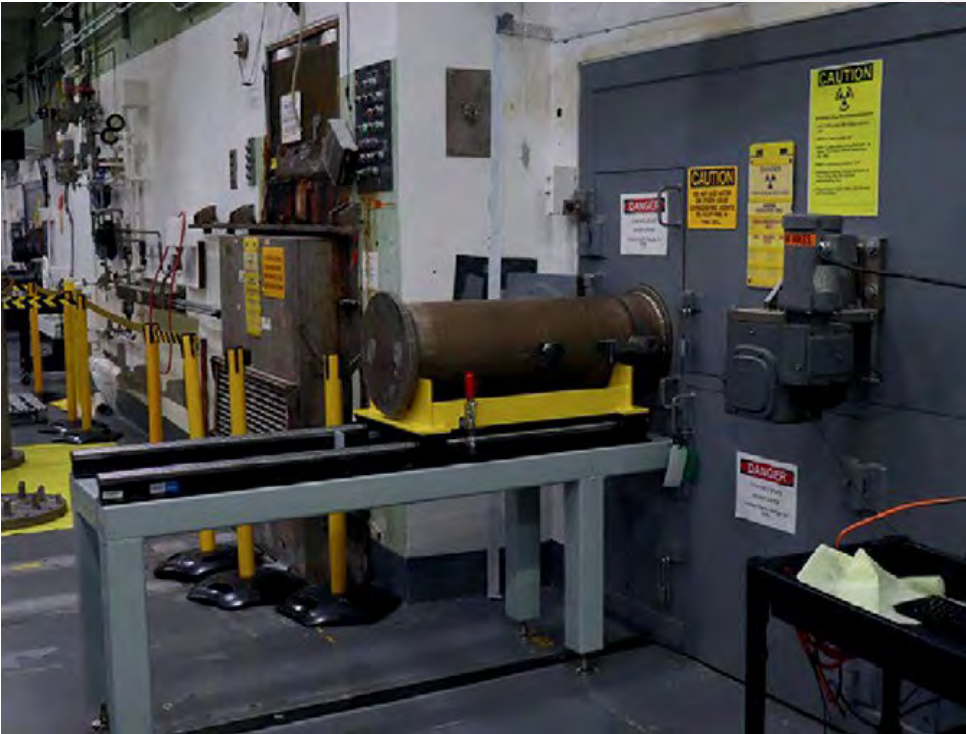
Figure 25. Uranium-233 canister within a transfer cask being loaded into a hot cell at Building 2026.
