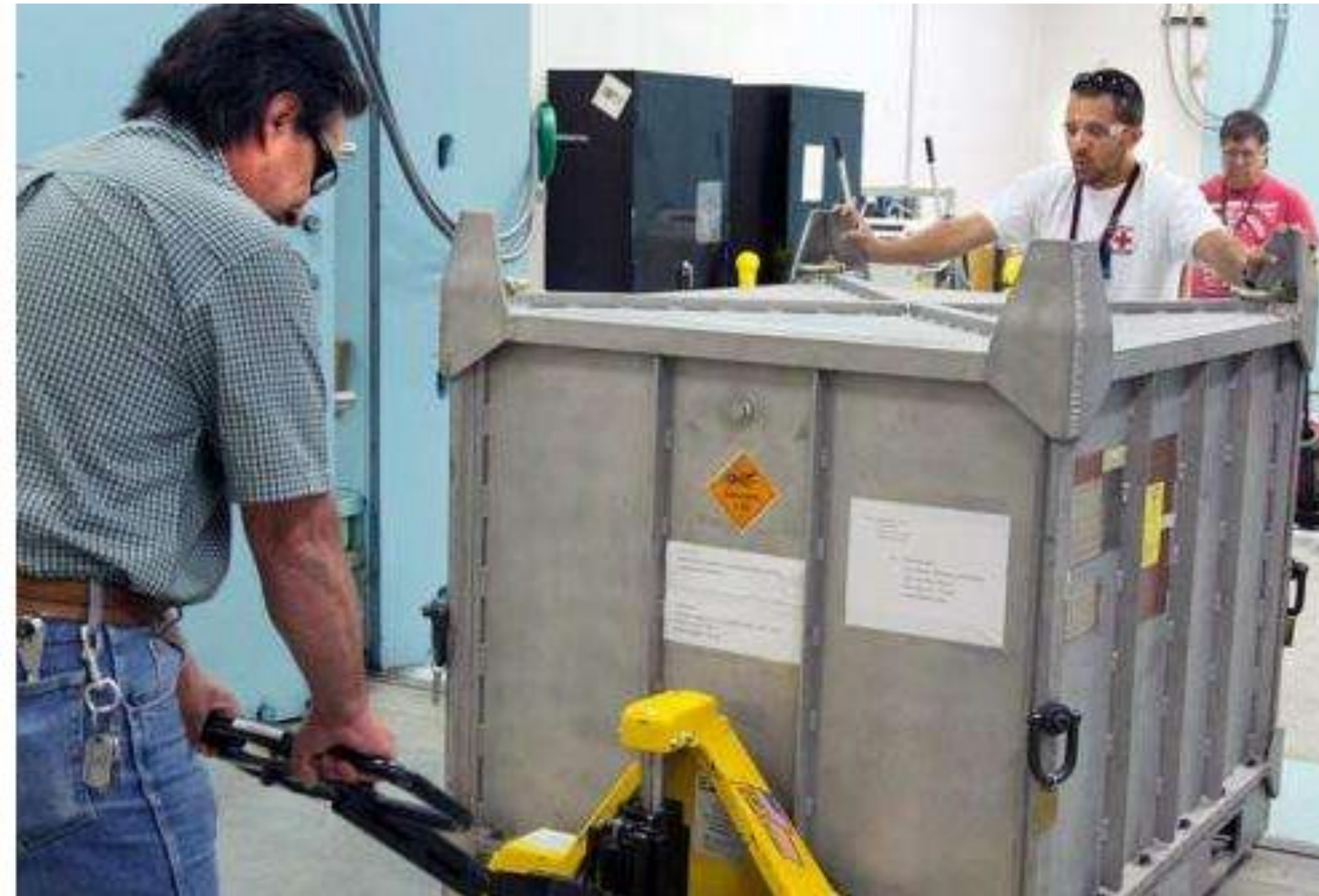
Shipping container for subcritical experiments involving radioactive materials and high-explosives. 11
