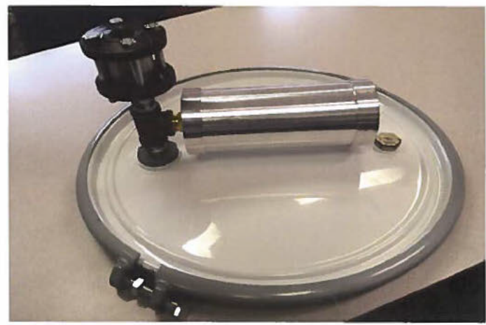
A HEPA filtration system will be installed on the RNS drums.
