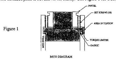
A loaded MCO weighs approximately 20,000 lbs, but the safety class Load Cell Verification System (LCV) high limit in the MCO Handling Machine (MHM) is 25,797 lbs and the high-high limit is 28,220 lbs. Assuming an MCO became stuck in a CSB tube and the first LCV limit failed, pulling on an MCO's pintel would stretch the MCO wall at the area in tension by approximately 38 millionths of an inch, as shown in Figure 2.
