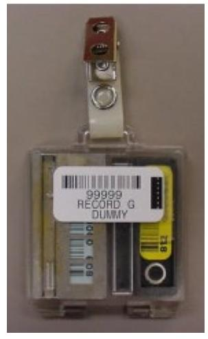
Figure 15. Thermoluminescent Dosimeter to Monitor External Radiation Dose
