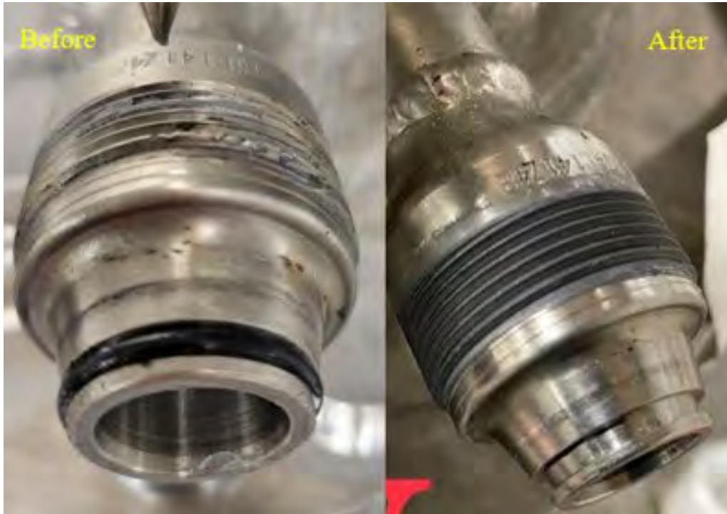
Figure 12. Tank Side Cesium Removal ion exchange column threaded connectors before and after repair.
