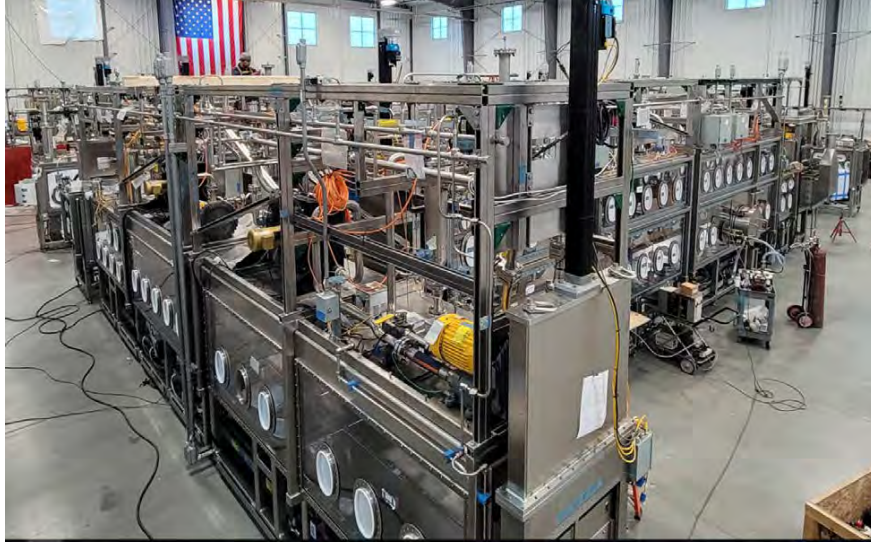
Figure 21. Glovebox line manufactured at a vendor facility.
