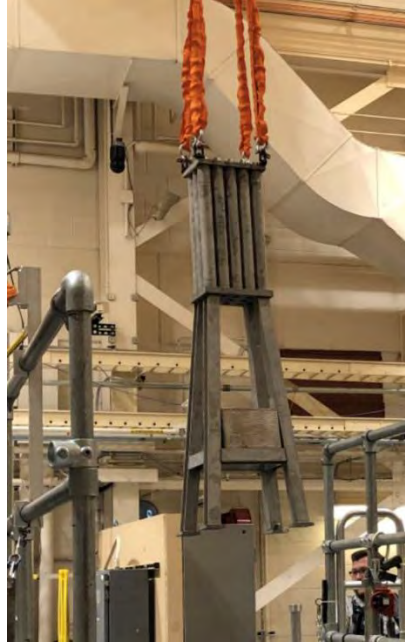
Figure 8. Annular Core Research Reactor fuel element rack lifted over the reactor pool.
