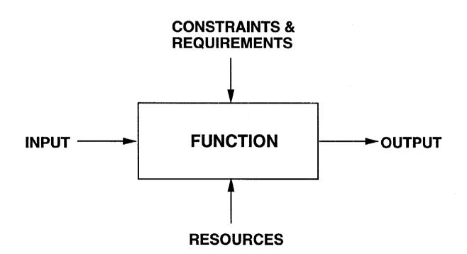
The Function operates on the Input with the provided Resources to produce a desired Output that meets the Constraints and Requirements.
