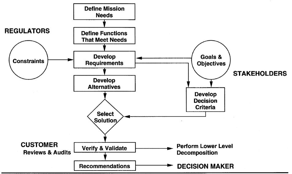
The LLW mission was decomposed into a set of functions that are necessary and sufficient to accomplish the mission. These functions were evaluated to determine an appropriate functional level for each function based upon the "functional value system" described above. The functional decomposition was performed by a team of Headquarters and Field Office Staff on a very accelerated schedule and must be considered conceptual in nature.
