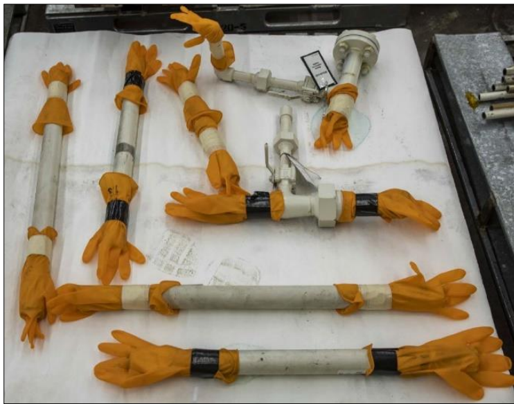
Figure 6. Machine Coolant Piping Capped with Rubber Gloves
