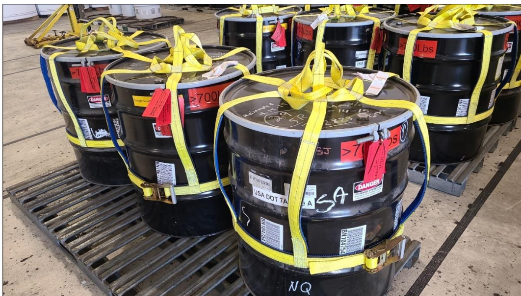
Figure 15. Lid Restraints on Drums with Flammable Gas
