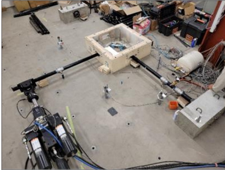
Figure 3. Test Apparatus for LANL's Plutonium Facility Fire Suppression System Fittings
