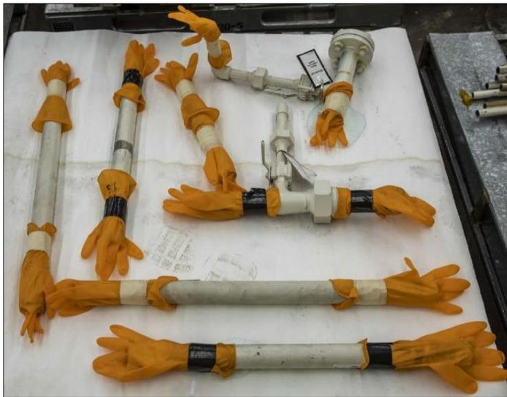
**Figure 6.** *Machine Coolant Piping Capped with Rubber Gloves*
