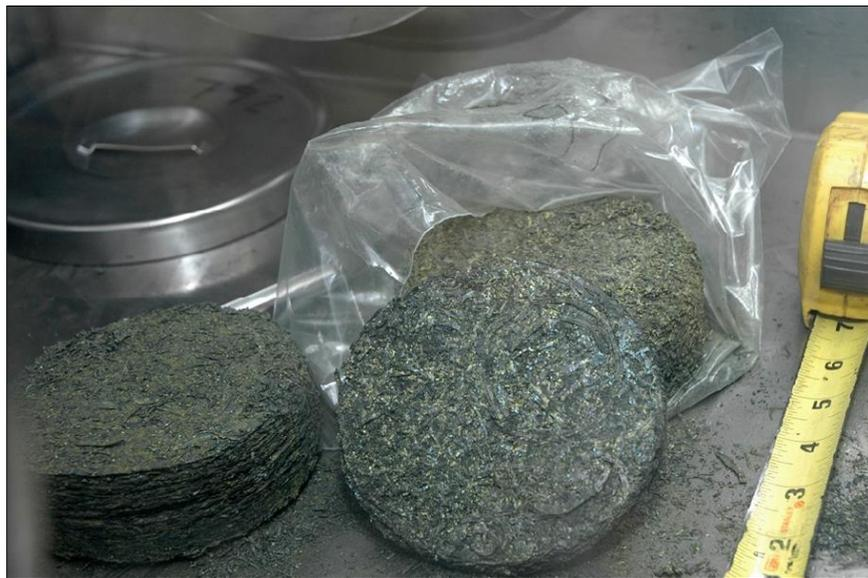
**Figure 7.** *Uranium Chip Briquettes*
