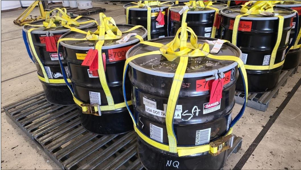
**Figure 15. Lid Restraints on Drums with Flammable Gas**
