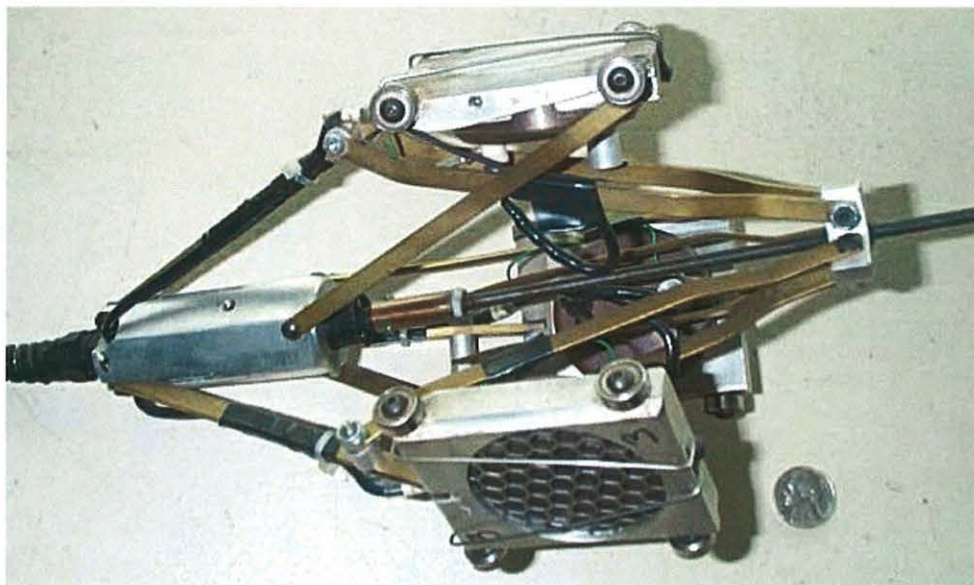
Figure 11: Example of Expanding Pipe Crawler
