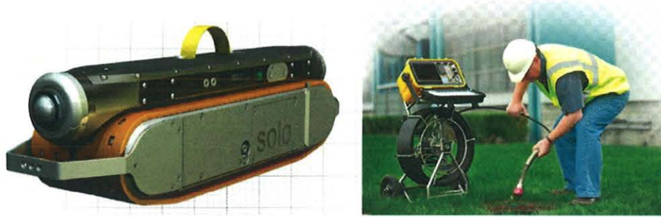
Figure 6: Typical Visual Inspection (ROV – Left, Borescope – Right)
