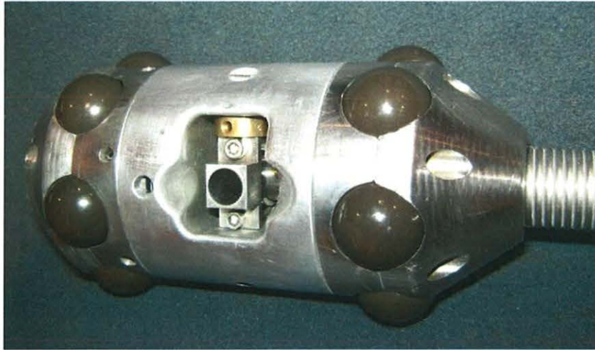
Figure 10: Example of Push Style Ultrasonic Probe
