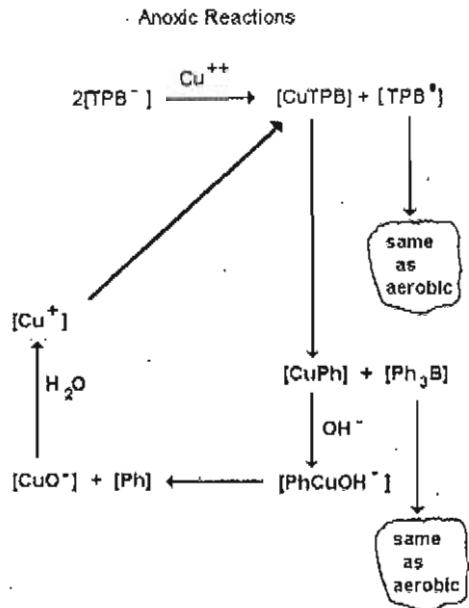
**Figure A-2. Anoxic Decomposition Reaction Scheme**
