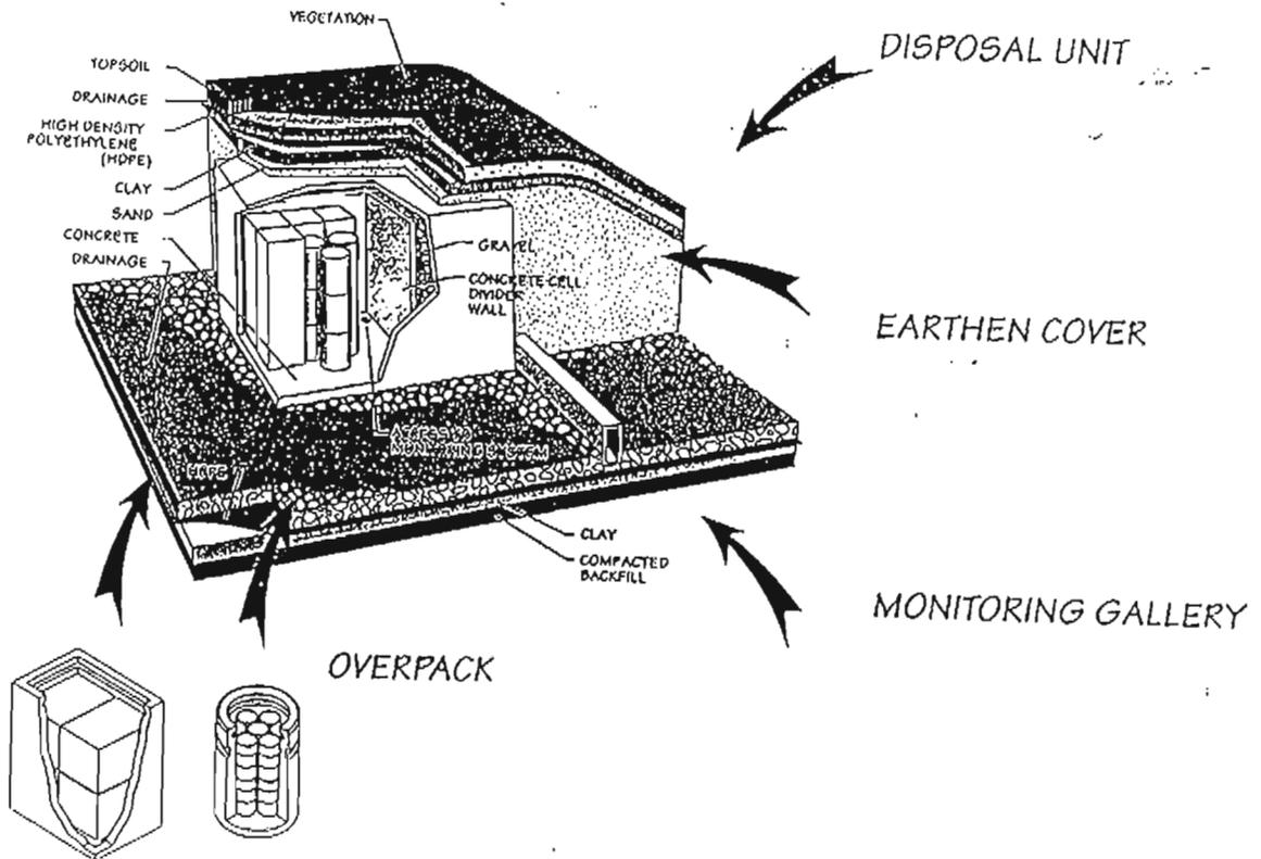
Figure C-4: Earthen-Covered Abovegrade Vault Disposal Facility<sup>64</sup>
