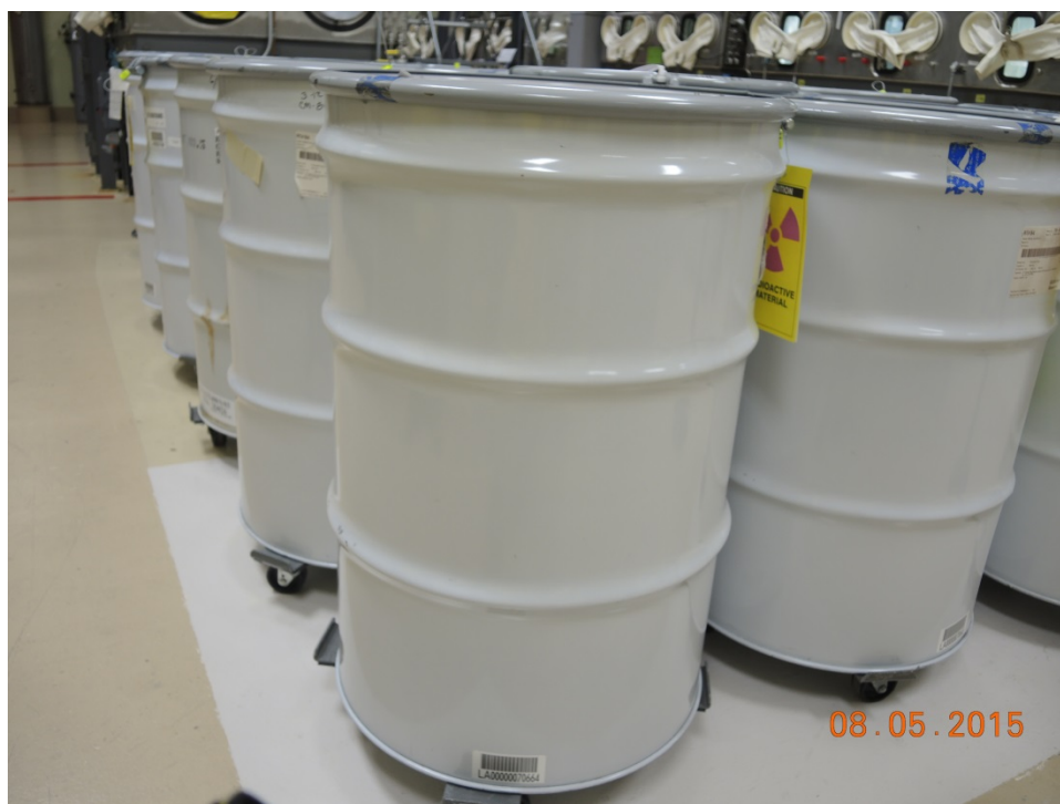
Figure 6: MAR contained in transuranic waste drums and staged in an operating laboratory.
