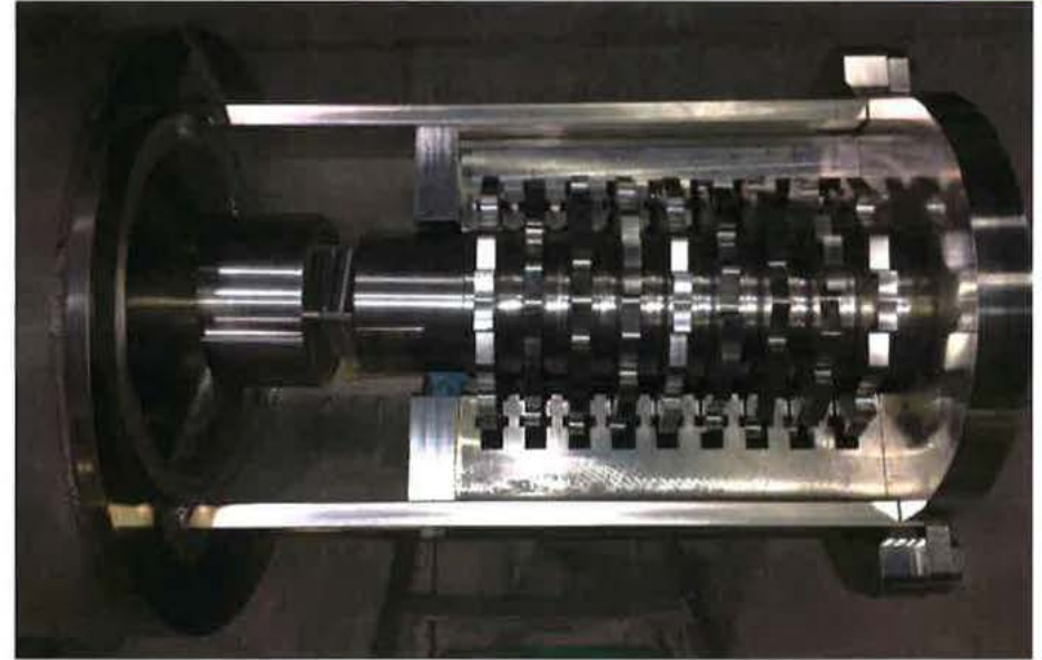
Prototype Auger-Grinder currently being tested.
