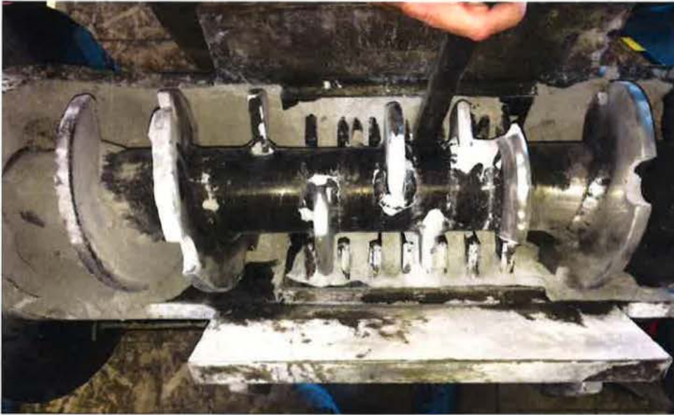
Auger-Grinder used in the May 2016 simulant run.
